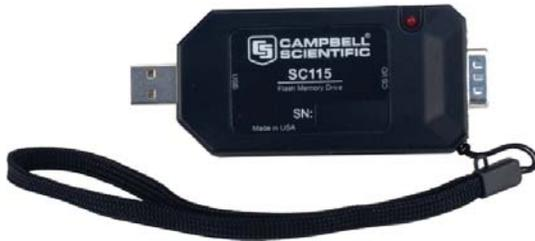
The SC115 is a light-weight, portable instrument that fits in a pocket allowing easy transport between the datalogger and PC.
